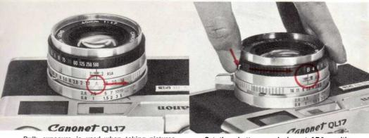
Bulb exposure is used when taking pictures with long time exposures.
